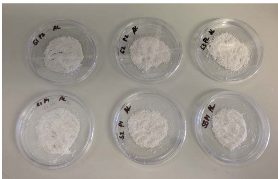
Figure 4.2: Example of sample pre-treatment by incubating soil with equal amounts of CaCO 3
