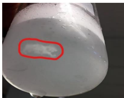
Figure A1.2: Precipitation of sample (AZT and TDF) when less than 10ml of the organic solvent (ethyl acetate and acetone) was used.
