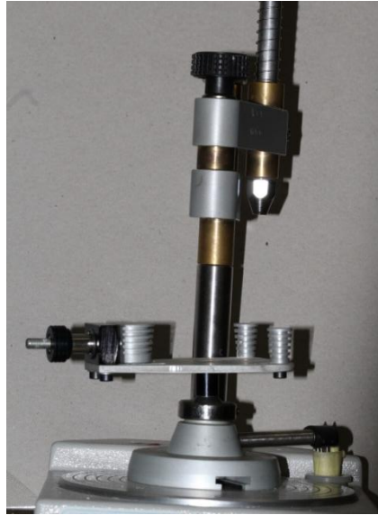
Figure 15: Surveyor used to align the teeth parallel (Dentalfarm, Torino, Italy)
