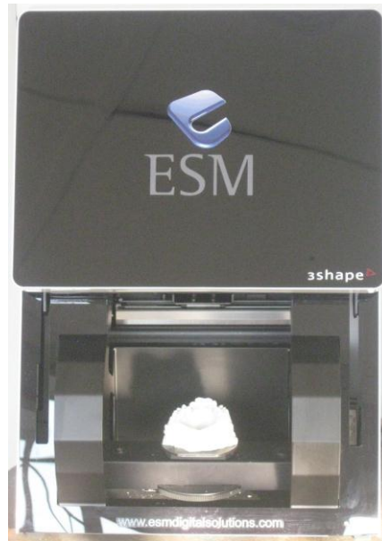
Fig 8. Plaster model in 3Shape R700™ scanner before being scanned.
