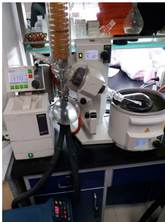
Figure 2.6: Vacuum rotary evaporator, which was used to concentrate the filtered solutions of medicinal plants.
