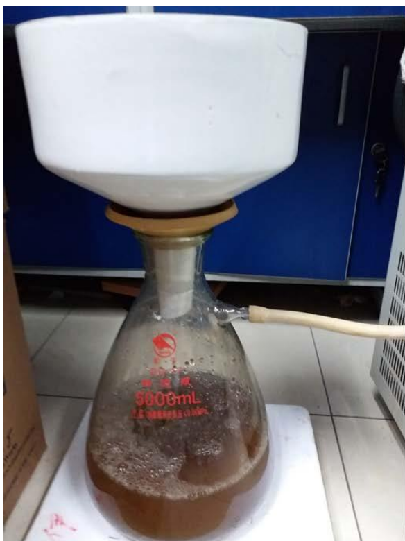
Figure 2.5: Suction filter was used to filter the solutions using the Whatman No.4 filter paper.
