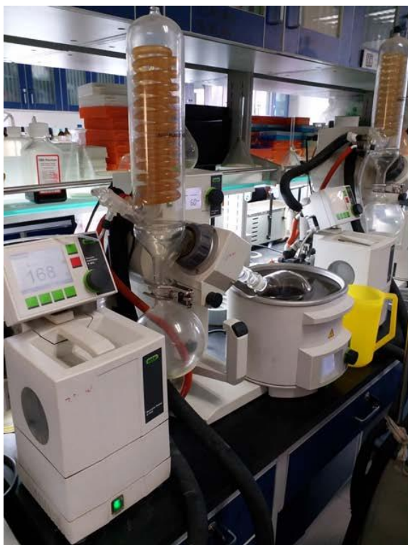
Figure 2.6: Vacuum rotary evaporator, which was used to concentrate the filtered solutions of medicinal plants.
