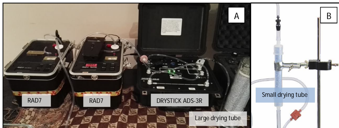
Figure 3-6: DURRIDGE manufactured components to reduce RAD7/s relative humidity (RH): DRYSTICK ADS-3R (A), large laboratory desiccant drying tube (A) and small desiccant drying tube (B).
