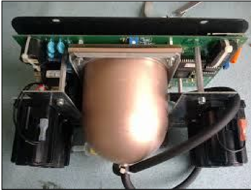
Figure 3-2: Inside components of RAD7 detector (side view) with the detection chamber visible in the centre. (Tan et al., 2014).
