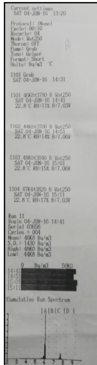
Figure 3-5: Print-out of radon-in-water activity concentration measurement results (four recycles), measurement parameters (Relative Humidity (RH), detector chamber temperature and battery voltage (B)) and cumulative run spectrum making use of the infrared-printer (see figure 3-1).
