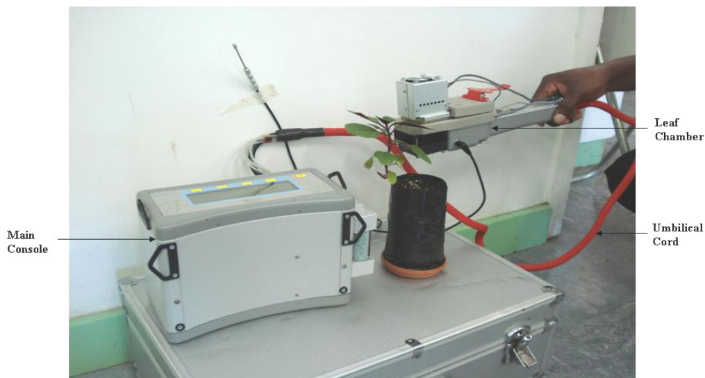
Figure 3.1: The physical components of an infra-red gas analyzer (IRGA). The device is a portable, field-use piece of equipment designed to measure plant leaf environments and their associated physiological processes. It comprises of the main console and the leaf chamber connected to each other with an “umbilical” cord. The main console contains a keypad, a display and a microprocessor-controlled operating system with a signal conditioning air supply unit and a data card. The leaf chamber has some movable jaws into which plant leaves are trapped during their physiological analysis and is also mounted with several sensors for detection and control of the chamber environment. (Figure from LC pro+ manual).
