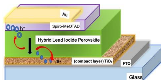
Figure 2.2 Illustration of charge transfer process in a hybrid organic-inorganic solar cell
