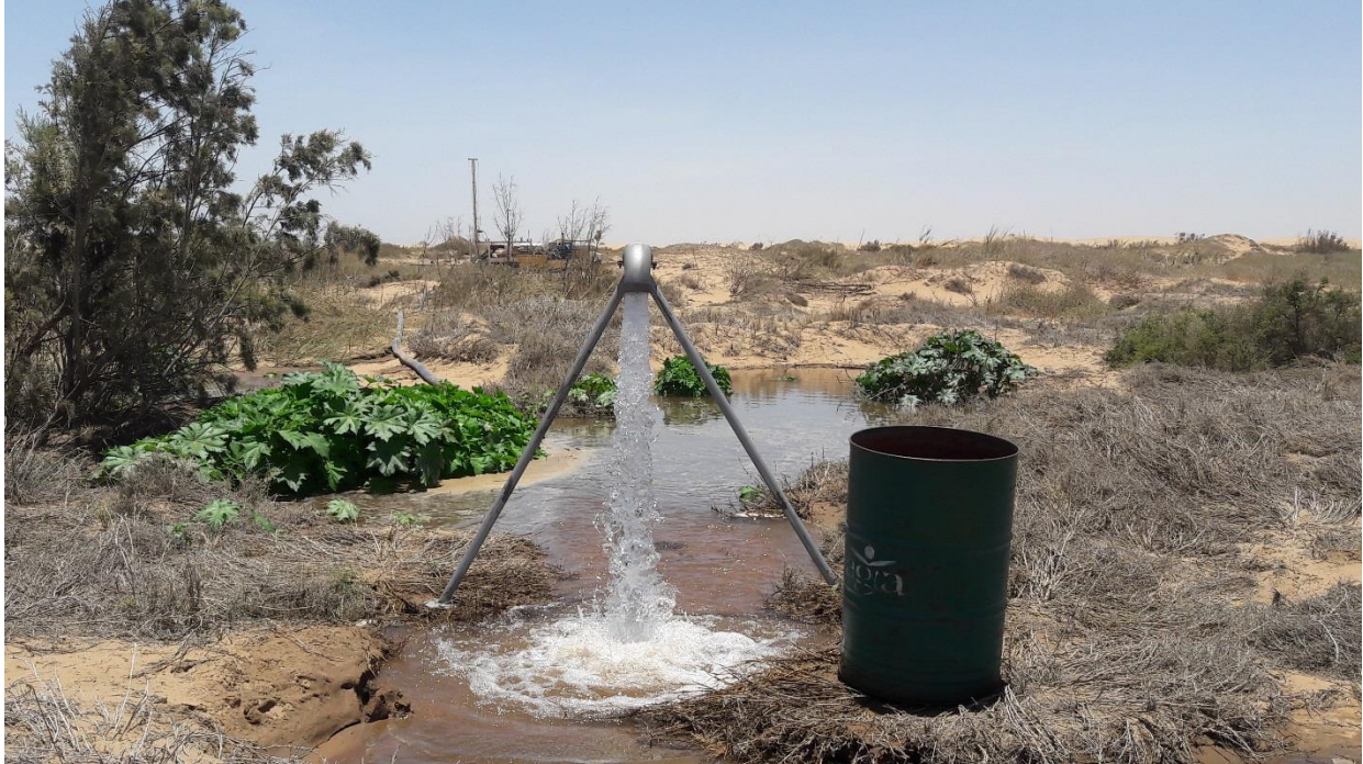
Fig. 2.4 Picture taken during CD test on borehole WW100292 at Dorop South
