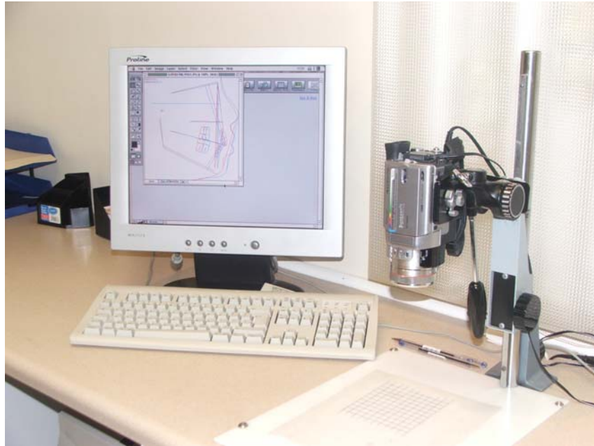
Figure 12. Digitizing apparatus consisting of a computer, a video camera and the Quick Ceph Imaging© software package.
