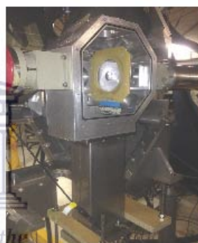
Figure 5: A double-sided (CD-type) S3 silicon detector placed upstream in the AFRODITE chamber during the RE measurements with ^{40}\text{Ar} beams last April 2015.
