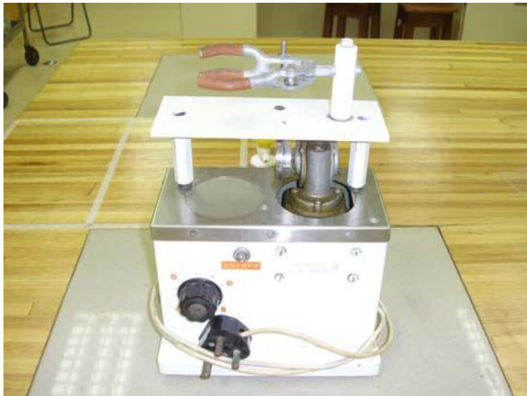
Figure 4. 2: Apparatus for density measurement
