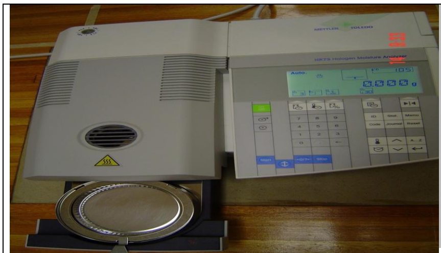
Figure 4. 4: HR73 Halogen moisture analyzer.
