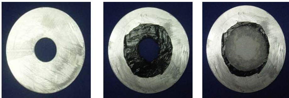
Fig. 1: Prepared membrane adhered on a support
