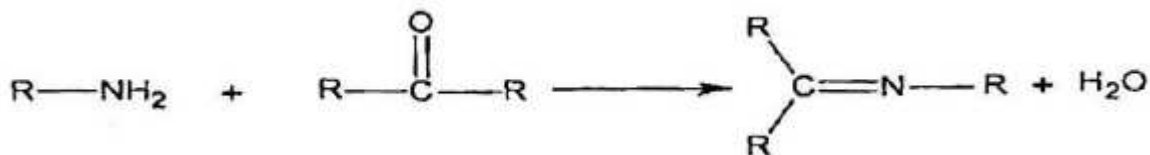
Figure 3-1: Scheme of Schiff base ligand synthesis
