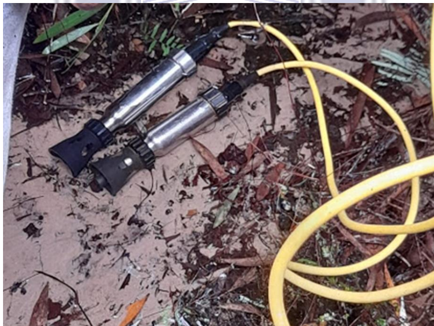
Figure 4.6: General chemical parameter measurement in-situ using YSI handheld multiparameter meter
